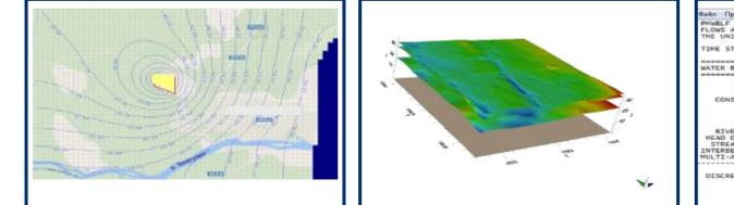
Setting of initial parameters (conditions of occurrence of aquifers and impermeable horizons, boundary conditions, porosity and permeability properties) Creating a conceptual model
